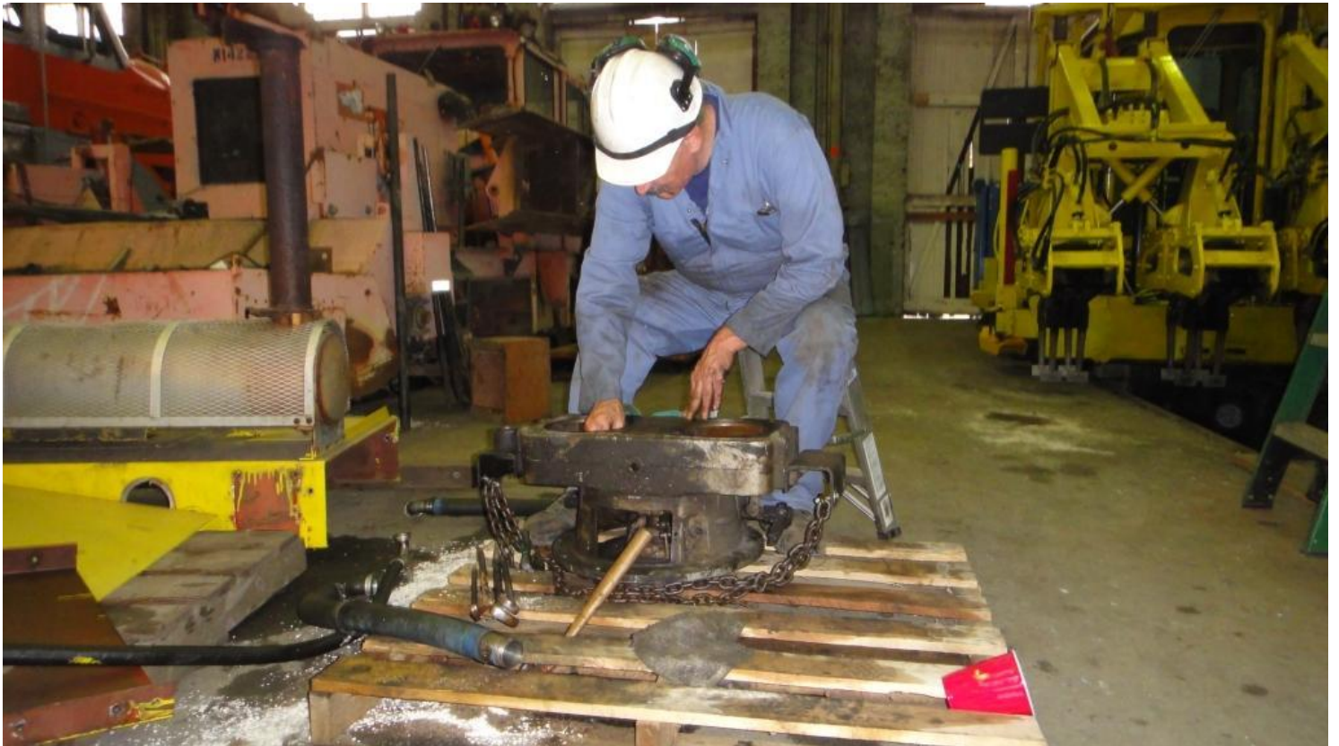
Fred working on the rebuild of the gear-box of the Tie Shear
